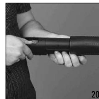
erating handle (Fig 14). One cartridge will be released from the magazine tube and it will rest on top of the carrier. Press the bolt release latch so the bolt can move forward, chambering a cartridge from the carrier (Fig 12).
