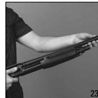
the muzzle, sliding it off of the magazine tube until it is completely removed (Fig 24).
