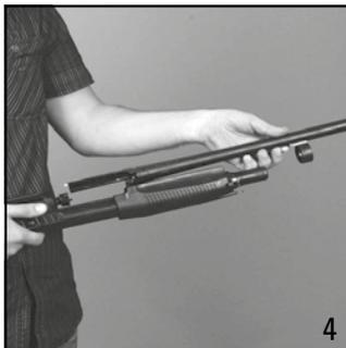
5. Screw the magazine cap (clockwise) onto the front of the magazine tube (Fig 7A), finger-tight. Make sure that the sling swivel is properly seated and centered on the magazine cap (Fig 7B) and the barrel is firmly seated.
