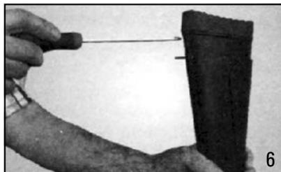
After the upper receiver separates, loosen the bolt two or three more turns. Gently tap the extension to further separate the upper receiver from the buttstock. You will note an expanding gap as you do this [Fig. 7b]. When the gap is around 1 inch / 2,5 cm remove the upper receiver retention bolt and washer.
